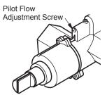
Figure 17 - Piliot Flow Adjustment Screw
